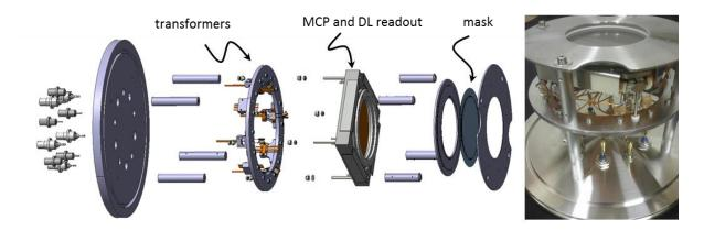
Fig. 1: sketch of the MCP and its RoentDek delay-line readout (left) and mounting (right)
