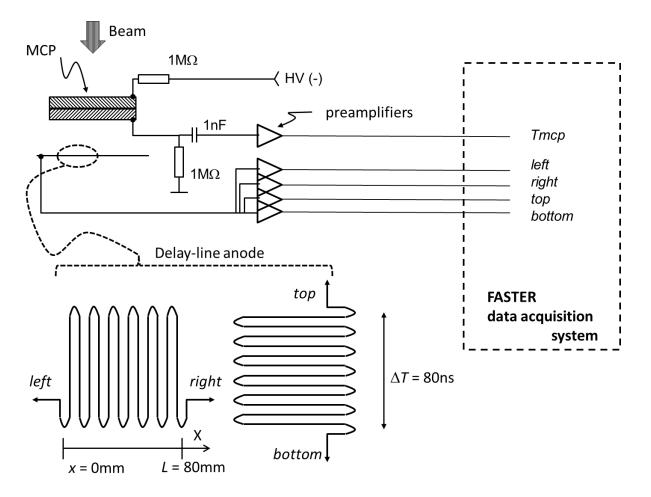
Fig. 3: Connecting of the MCP + delay-line readout to a FASTER data processing and acquisition system
