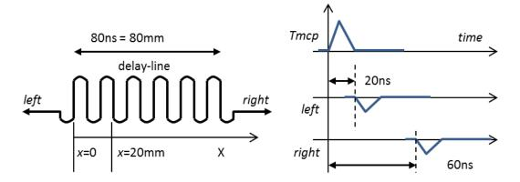
Fig. 2: MCP & delay-line signals vs particle position
