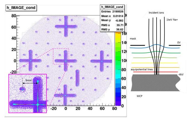
Fig. 4: raw image of bottom-top vs left-right (pulse times measured by the mean of FASTER CFD)
