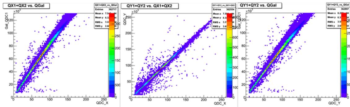
**Fig. 6: event consistency check by the mean of charge correlation**
