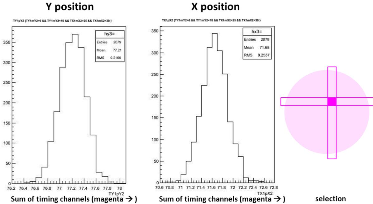
**Fig. 7: indirect measurement of localization uncertainty**
