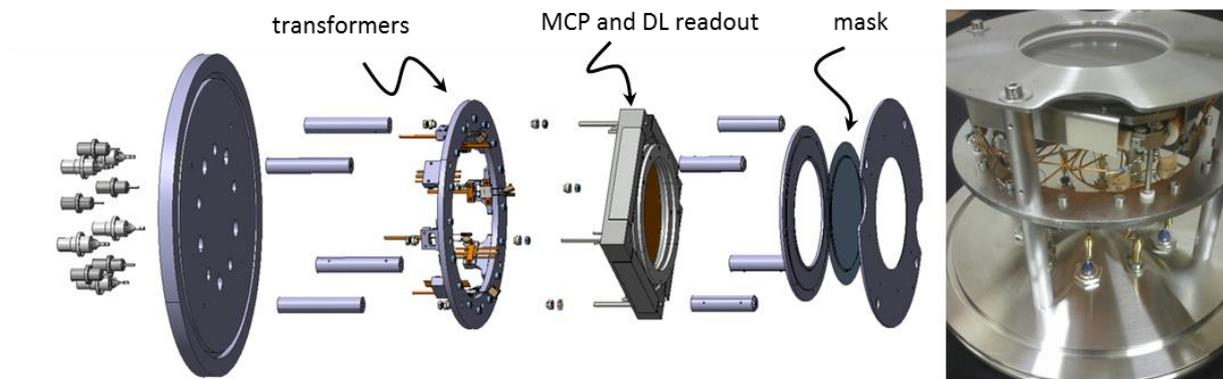
**Fig. 1:** sketch of the MCP and its RoentDek delay-line readout (left) and mounting (right)
