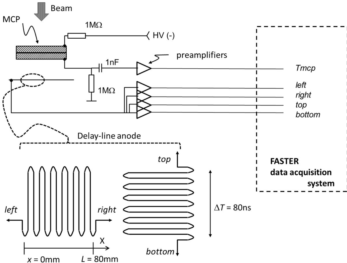
**Fig. 3: Connecting of the MCP + delay-line readout to a FASTER data processing and acquisition system**
