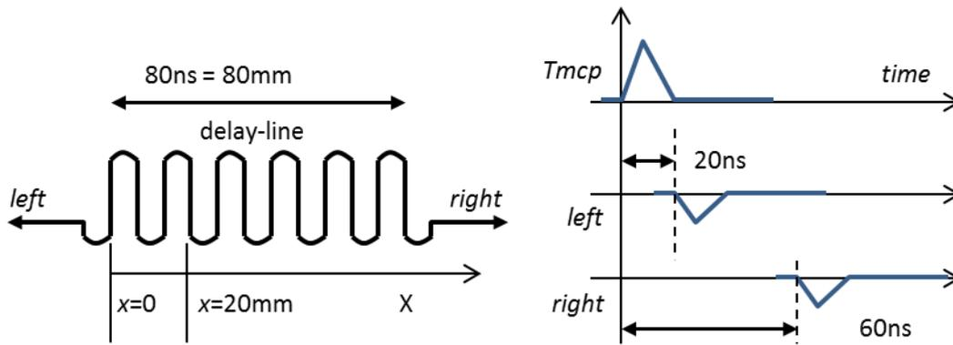
**Fig. 2: MCP & delay-line signals vs particle position**
