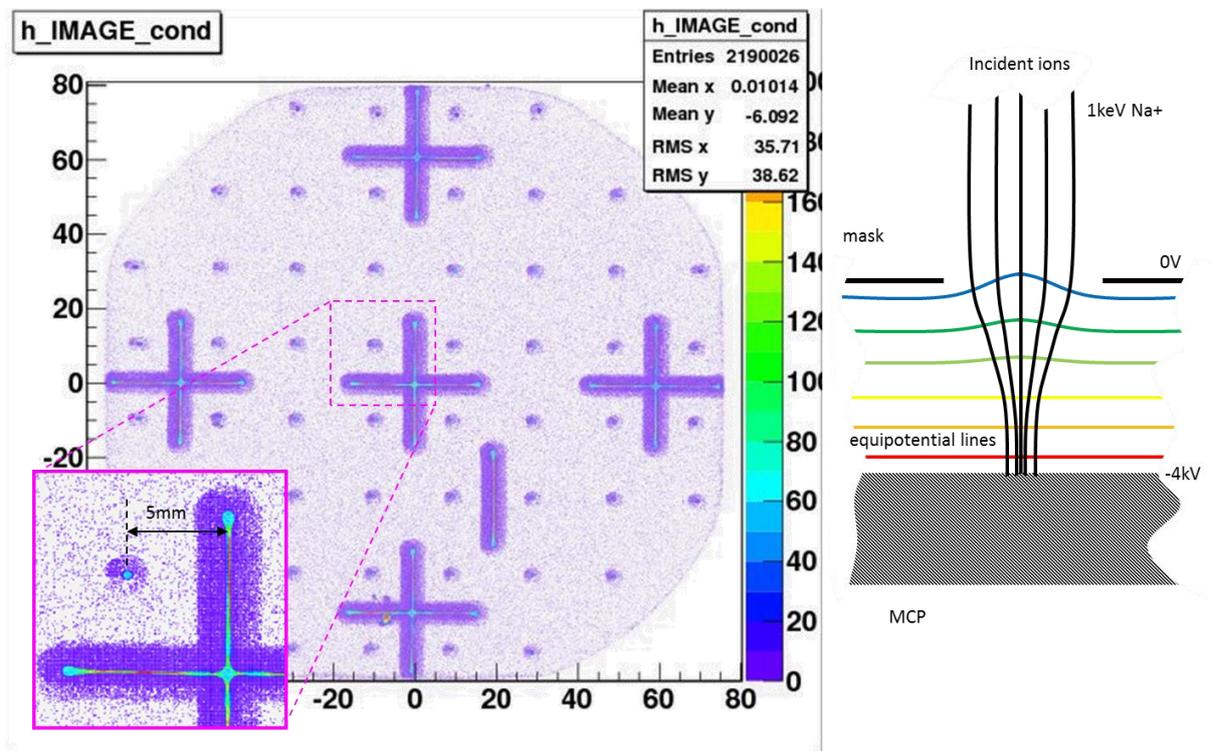
Fig. 4: raw image of *bottom-top* vs *left-right* (pulse times measured by the mean of FASTER CFD)
