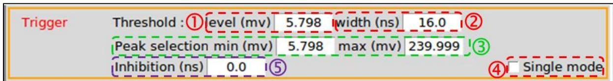
Figure 20: parameters of the threshold discriminator.
