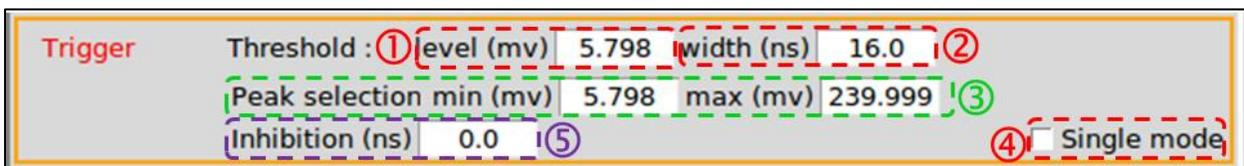
Figure 20: parameters of the threshold discriminator.
