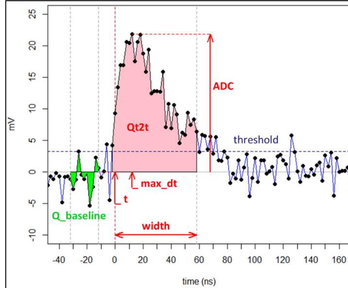
Figure 27: Information from QT2T data. The “saturated” flag is not represented.
