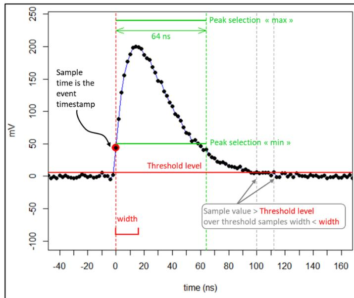
Figure 21: The first pulse, which has crossed the threshold level is detected. The following ones are not, thanks to a judicious value of the “width” parameter.
