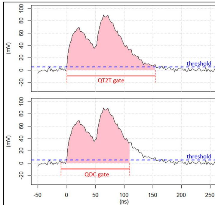
Figure 1: Difference between the QT2T gate and the QDC gate : the QT2T gate expands according to the time width of the pulse
