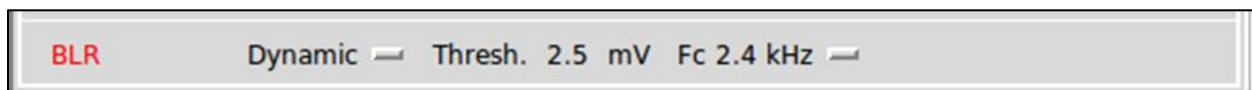
Figure 32: 2 of the 3 parameters of the dynamic BLR shaper: BLR threshold and cut-off frequency.
