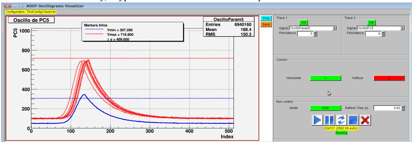
User gets thus expected standard oscilloscope functions to select signals, set cursors on axis and select a persistence value for both signals.
